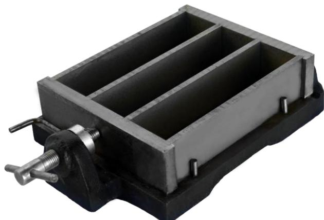
Cement Cubic Grinded Mold, 50x50x50mm, 3 gang, Cast Iron Model: 2221010
